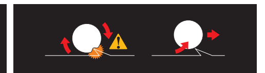
Weaker shells may deform on impact, possibly catching on obstacles or reducing their ability to slide over uneven surfaces.
