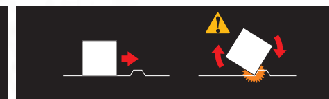
Exaggerated shell shapes that address ventilation or aerodynamics may reduce a helmet's ability to avoid digging in or snagging that may allow more impact energy into the helmet or may cause high rotational force.
