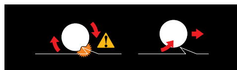
Weaker shells may deform on impact, possibly catching on obstacles or reducing their ability to slide over uneven surfaces.
