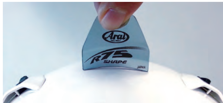
The Arai R75 gauge in use. Wherever the two ends of the gauge are touching, the helmet is conforming to the R75 shape concept.
